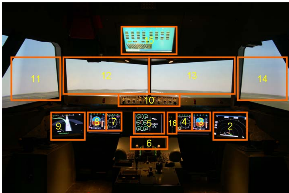
Figure 1. Picture of the generic cockpit simulator including the various areas of interest.
